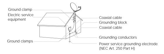
Note: If the Satellite/Antenna cable is grounded correctly (as specified above), connecting it to the DIRECTV Digital Satellite Recorder will properly ground the recorder. The recorder must be properly grounded before you connect it to a telephone line, and it must remain grounded thereafter.
